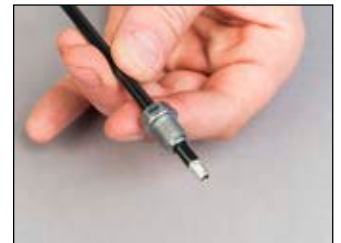
Mounting the union nut
