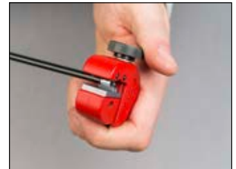
Positioning of line to scrape the covering
