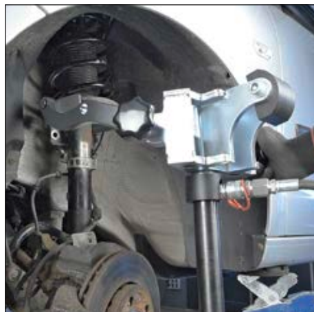
2. Pre-tension springs directly on the vehicle
